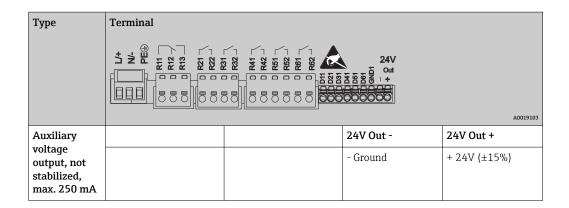
If the auxiliary voltage is to be used for the digital inputs, the **24 V out** - terminal of the auxiliary voltage output must be connected with the **GND1** terminal.
