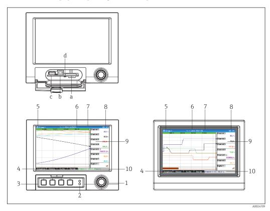
Device front (left: version with navigator and front interfaces; right: version with stainless steel front and touchscreen)
