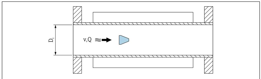
$D_i$  Internal diameter of measuring tube (corresponds to dimension K → 52)
