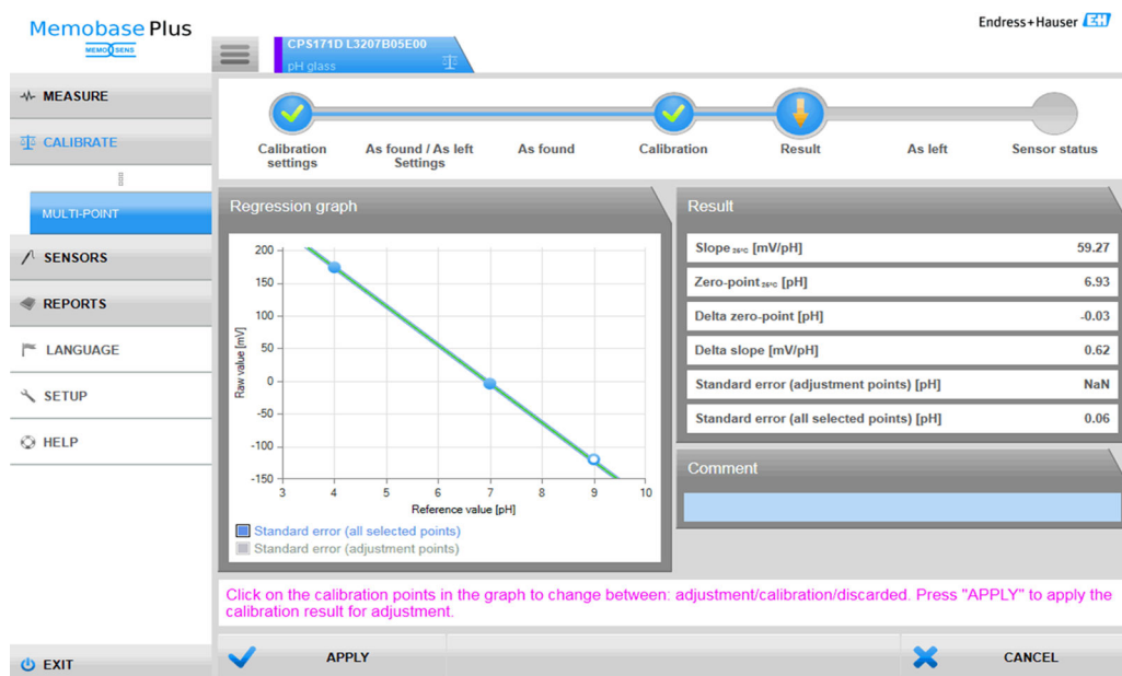
4 Multipoint calibration ("Advanced diagnostics" license): buffers 4 and 7 selected as the adjustment points, buffer 9 as the calibration point
