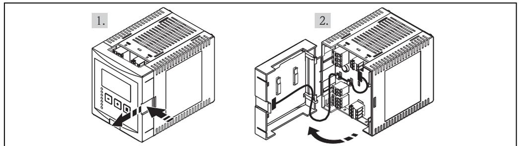
The catch can be unlocked by slightly pressing onto the clip. Then, the cover of the terminal compartment can be opened.
