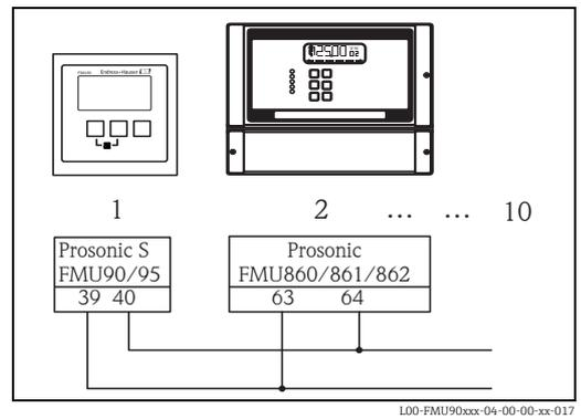
**Connection of the separate display and operating module**
